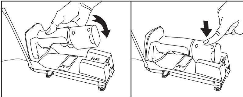
Rapid flashing indicates that charging is taking place. Rapid charging occurs when the battery temperature is between 10°C (50°F) and 46°C (115°F), and/or voltage of the battery is between 2.0 and 3.2V. Charge time is less than 4.2 hours. Rapid charge ends with the battery at approximately 90 to 95% capacity. The CHARGE LED remains on steady when trickle charging or after the charge cycle is complete.
